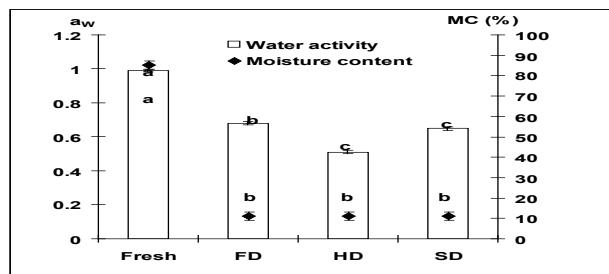
**Figure 1.** Water activity and moisture content of fresh and dried chilli using different drying methods.
